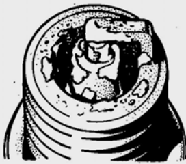
White deposits and damaged porcelain insulation indicating overheating
