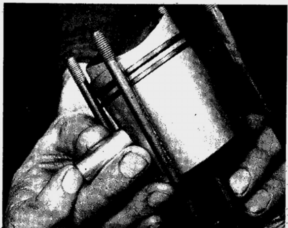
32.2 Gudgeon pin should press into position
