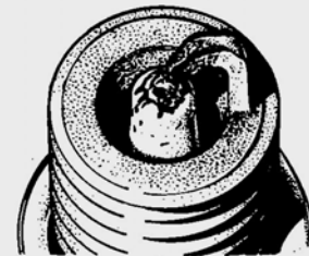
Electrodes burnt away due to wrong heat value or chronic pre-ignition (pinking)
