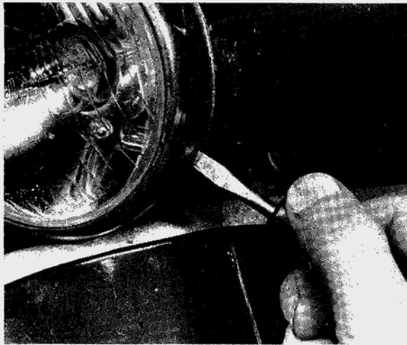
6.1 Headlamp rim and reflector unit is retained to shell by two screws
