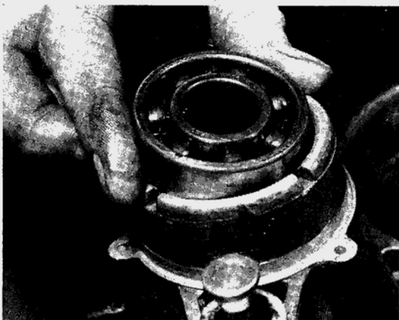
29.1a Warm casting before replacing bearing
