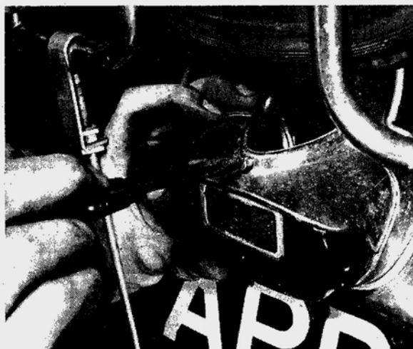
9.1 Single screw retains rear lamp cover
