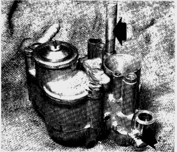
8.2 Throttle stop and pilot jet adjusting screws
