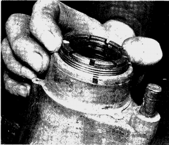
29.1b Tighten bearing retainer fully
