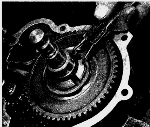
29.7c . . . . circlip that retains assembly in position
