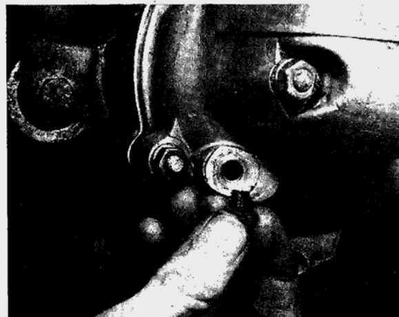
38.3 Make sure gearbox is refilled before replacing filler plug
