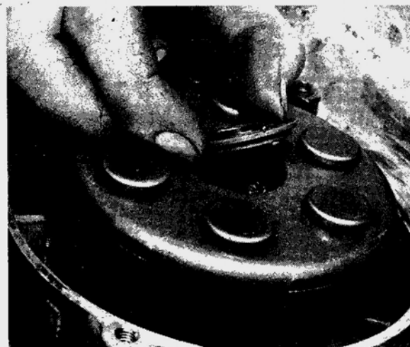
30.2 Replace thrust plate in centre
