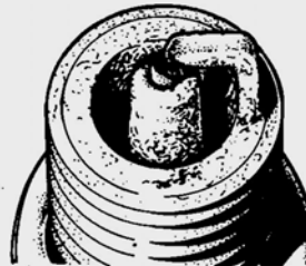
Mild white deposits and electrode burnt indicating too weak a fuel mixture
